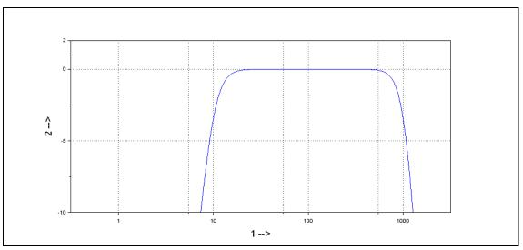
Fig. 6: Typical frequency response 10 Hz–1000 Hz
