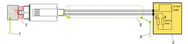
Fig. 11: Alternative earthing concept
