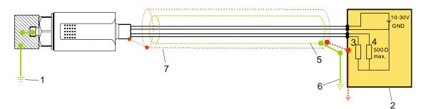
Fig. 10: Standard earthing concept
