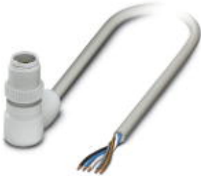
Sensor/Actuator cable, 5-position, PP-EPDM halogen-free, Gray RAL 7035, Plug angled M12, A-coded, on Free cable end, Cable length: 10 m, Hygienic design, with plastic knurl
