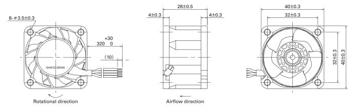
Fig. 2 Dimensions of the San Ace 40L 9LG type (Unit: mm)
