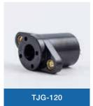
Conductors: 5 Conductor Type: Nickel-Plated BeCu Description: Flange Rear-Mounted Jack; with an extra contact added in a normally open circuit with the #1 contact. Insertion of a 4-conductor plug closes the #1-5 contact circuit.
