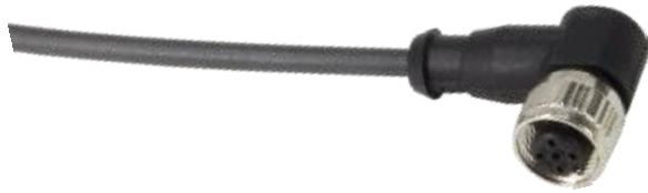
M12 3-pole Single Ended Overmolded Angled PUR Black
