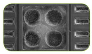
Solder points on PCB (magnification 11.25x)
