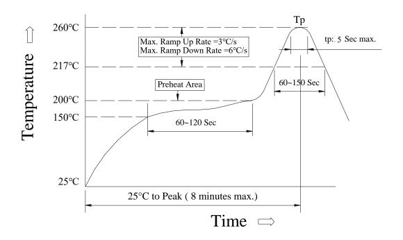
Reflow Soldering Method:
