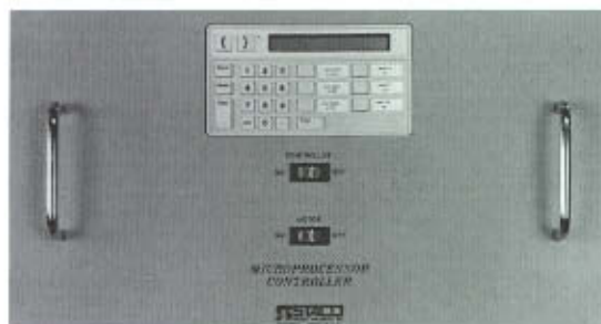
Rack Mounted Microprocessor Controller
