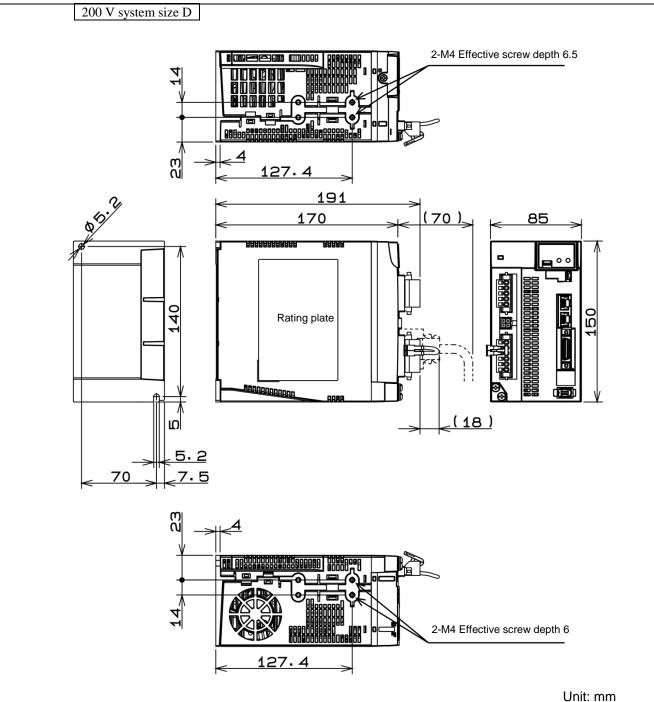
\* Do not use threaded screw holes that do not have description of dimensions.
