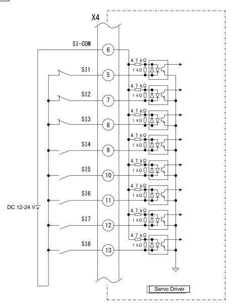
Functions SI1 to SI8 should be allocated by parameters. For details, refer to "Technical Document - Basic Functional Specifications -".
