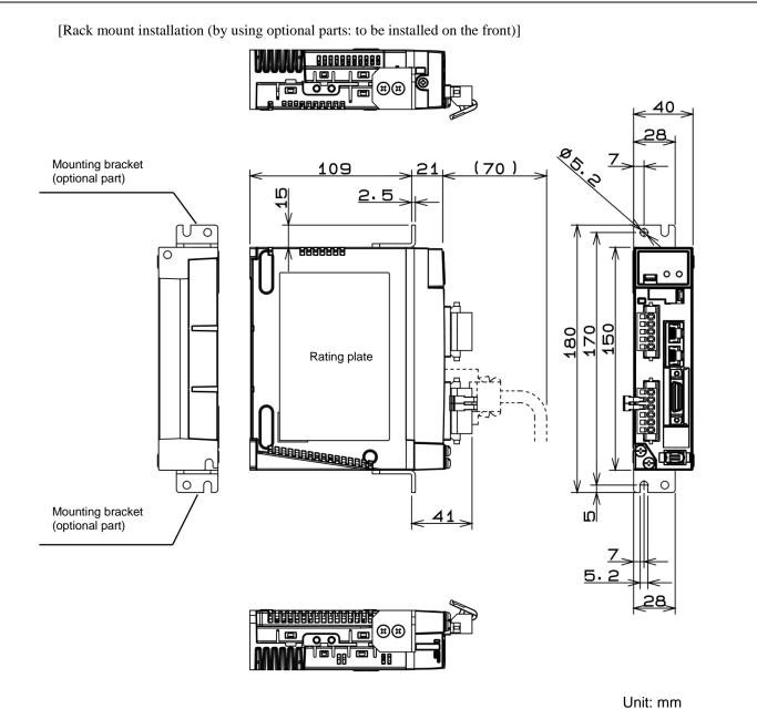
$\ast$  Do not use threaded screw holes that do not have description of dimensions.
