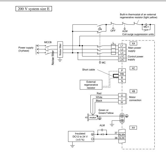
■ Connection of a regenerative resistor
