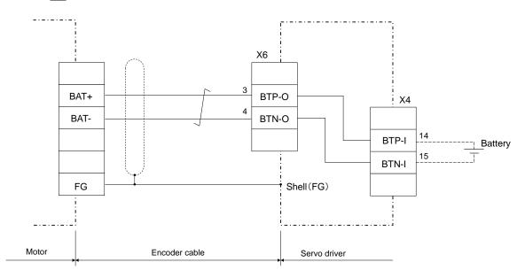
Note: When connecting the battery directly to the encoder connector on the motor side, do not connect anything to the 3pin and 4pin of the  $\underline{X6}$  connector.
