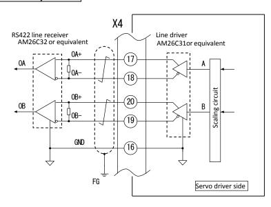
[1] Use an RS422 line receiver (AM26C32 or equivalent) to receive output pulse.
