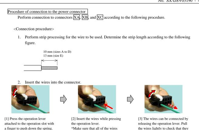
\*Make sure that all of the wires are inserted into the opening part of the spring.
