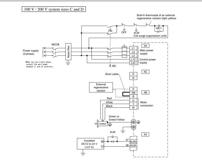
■ Connection of a regenerative resistor
