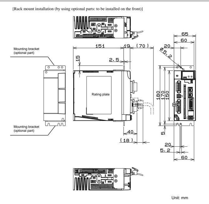
\* Do not use threaded screw holes that do not have description of dimensions.
