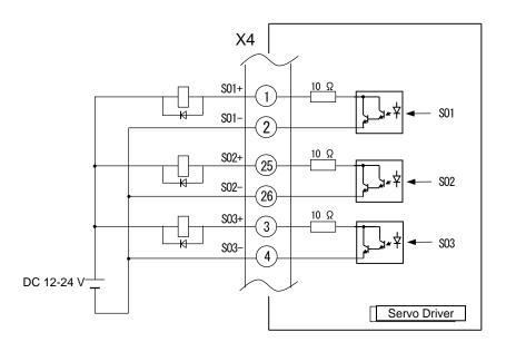
Functions SO1 to SO3 should be allocated by parameters. For details, refer to "Technical Document - Basic Functional Specifications -".
