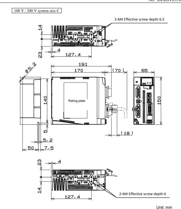
\* Do not use threaded screw holes that do not have description of dimensions.
