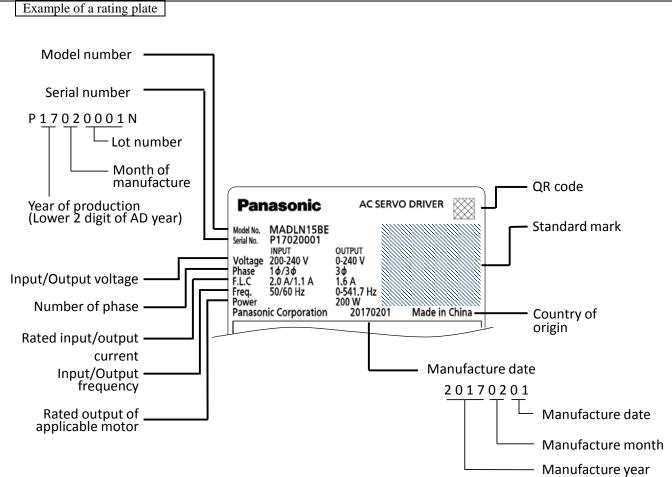
The values of the serial number part of the manufacturing number range from 1 to 33999. On the rating plate, it is indicated in four digits as in the format shown below.
