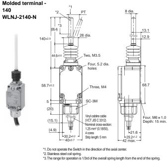
Note: Unless otherwise indicated, a tolerance of ±0.4 mm applies to all dimensions.
