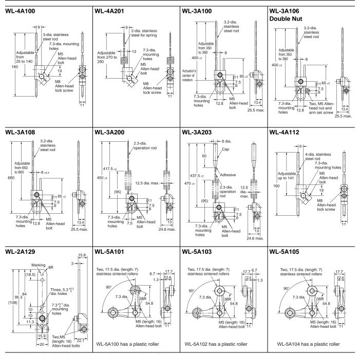
Note: 1. Unless otherwise indicated, a tolerance of ±0.4 mm applies to all dimensions.
