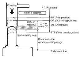
The Limit Switch may soon malfunction if the OT is excessive.
