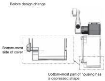
The line of the bottom-most face of the cover is 4 mm below the cover attachment screw and is long
