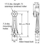
Note: Unless otherwise indicated, a tolerance of  $\pm 0.4$  mm applies to all dimensions.
