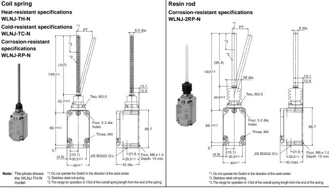
**Note:** Unless otherwise indicated, a tolerance of  $\pm 0.4$  mm applies to all dimensions.
