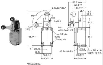
\*Plastic Roller (The WLCA32-041-N to WLCA32-044-N have stainless sintered rollers.)
