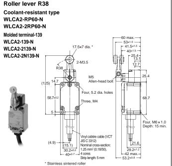
Roller lever R38 With operation indicator Coolant-resistant specifications WLCA2-RP60LD2-N WLCA2-RP60LD3-N WLCA2-2RP60LD2-N 60 max WLCA2-2RP60LD3-N 53±1.5 — - 41.5±1.5 17.5x7 dia. \* Molded terminal -139 WLCA2-139LD2-N WLCA2-139LD3-N WLCA2-2139LD2-N WLCA2-2139LD3-N (125) bolt Four, 5.2 dia. holes ф Three, M4 Four, M6 × 1.0
