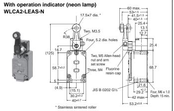
Note: The photo shows the WLCA2-LDAS-N model.
