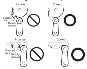
Appropriate force must be imposed on the actuator by the cam or dog in both rotary operation and linear operation. If the dog touches the lever as shown below, the operating position will not be stable.
