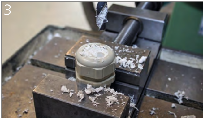
Taladro realizado Bore-hole executed
