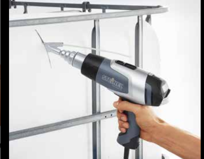
▲ Welding water tank HG 2320 E
