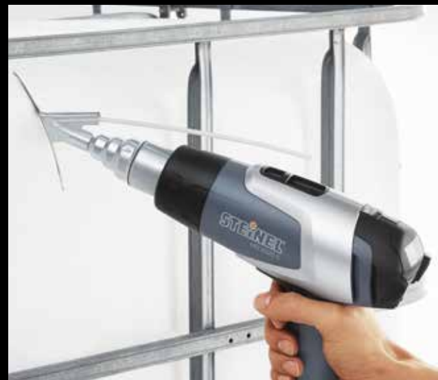
Plastic welding with a reduction nozzle.
