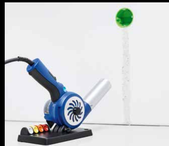
Drying plasterwork faster with hot air.
