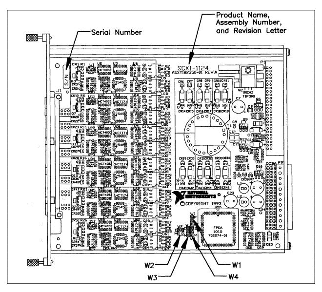
Figure 2-1. SCXI-1124 Parts Locator Diagram
