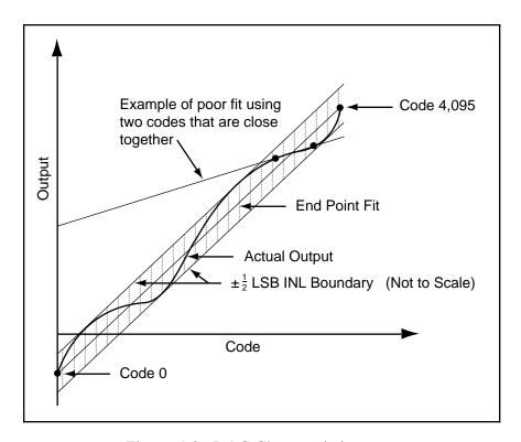
Figure 5-2. DAC Characteristics
