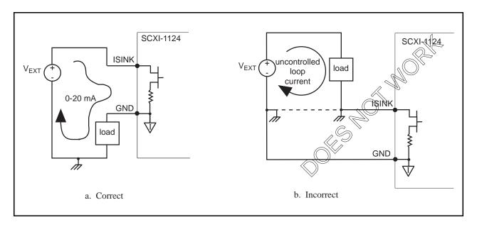
Figure 3-5. Current Loop Connection, Load and External Supply Both Grounded
