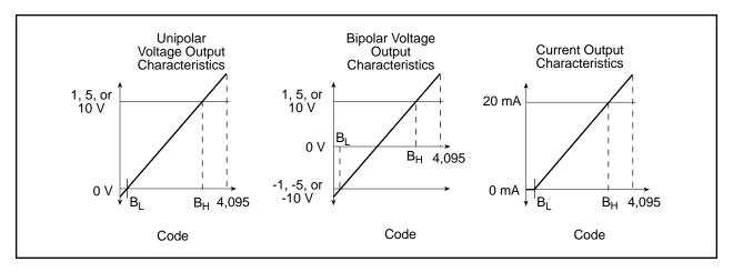
Figure 5-1. SCXI-1124 Output Characteristics
