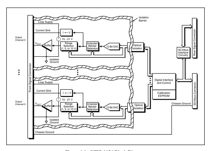
Figure 4-1. SCXI-1124 Block Diagram
