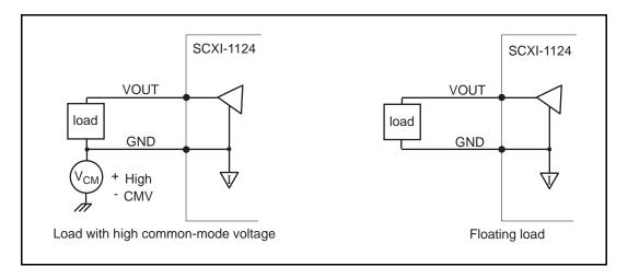
Figure 3-2. DAC Channel Connection as Voltage Output
