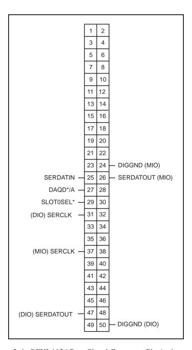
Figure 3-6. SCXI-1124 Rear Signal Connector Pin Assignments
