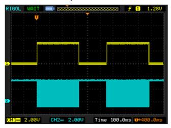
Channel 1 (yellow/top) – Pin #12 (DSW\_LED\_DRV) with external  $5k\Omega$  pull up resistor Channel 2 (light blue/2<sup>nd</sup> line) – Pin #11 (S4\_LED\_DRV) with external  $5k\Omega$  pull up resistor
