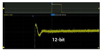
12-bit resolution shows you more details and less noise on the waveform.T3DS01204, T3DS01302A
