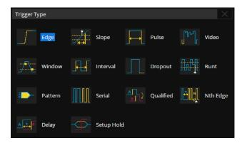
Edge, Slope, Pulse, Video, Windows, Runt, Interval, Dropout, Pattern, Qualified, Nth edge, Setup/hold, Delay, and serial trigger.
