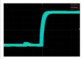
The oscilloscope utilizes a hardware-based Mask Test function, performing up to 14,000 Pass / Fail decisions each second. It is easy to generate user-defined test templates to provide trace mask comparisons, making it suitable for long-term signal monitoring or automated production line testing.
