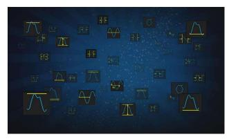
Parameter measurements include 4 categories: horizontal, vertical, miscellaneous, and CH delay providing a total of 50+ different types of measurements. Measurements can be performed within a specified gate period. Measurements on Math, Reference, and History frames are supported.
