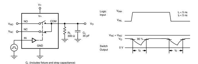
Figure 2. Break-Before-Make Interval
