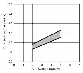
Switching Threshold vs. Supply Voltage
