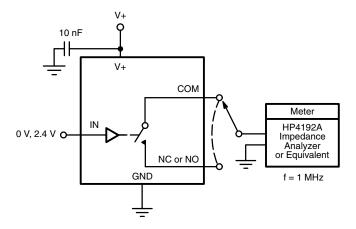
Figure 5. Channel Off/On Capacitance
