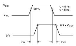
Logic "1" = Switch On Logic input waveforms inverted for switches that have the opposite logic sense.
