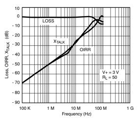
Insertion Loss, Off-Isolation, Crosstalk vs. Frequency
