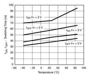
Switching Time vs. Temperature and Supply Voltage
