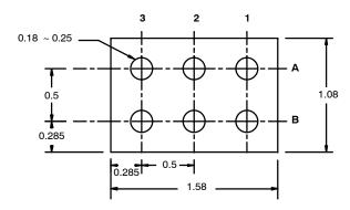
FIGURE 2. Outline of MICRO FOOT CSP & Analog Switch DG3000DB
