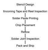
FIGURE 5. SMT Assembly Process Flow
