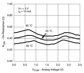
R<sub>ON</sub> vs. Analog Voltage and Temperature
