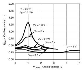
$R_{ON}$  vs.  $V_{COM}$  and Supply Voltage
