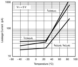
Leakage Current vs. Temperature
