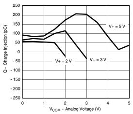
Charge Injection vs. Analog Voltage
