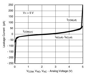
Leakage vs. Analog Voltage
