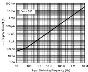
**Supply Current vs. Input Switching Frequency**
