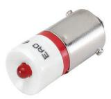
Illuminative colour Operating voltage 130 V DC +10% Operating voltage tolerance +10% % Operation current  $3 \text{ mA} \pm 15 \%$ Operation current tolerance ±15 % % Weight 0.002 kg Illumination colour Red 630 nm Dom. Wavelength Lumi. Intensity 120 mcd
