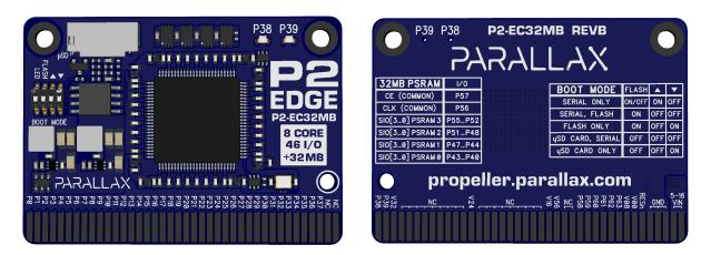
The P2 Edge Module with 32MB RAM is a simple way to get started with the Propeller 2 multicore microcontroller. In addition to speeding development, this module provides an optimal P2 building block for system integrators and designers to include in their products.
