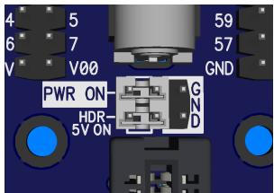
**PRO TIP: REMOVE THE HDR 5V ON JUMPER IF YOU ARE NOT USING THE 5V SUPPLY AT THE 2X6 WAY ACCESSORY HEADERS.** Doing so will reduce the risk of accidentally causing damage during experimentation; for example, should one of the 5V pins be accidentally connected to a signal or ground pin. All I/O signal pins are rated for 3.3V only!
