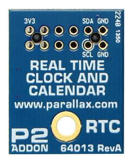
The P2 RTC Add-On Board provides a real time clock with calendar and alarm functionality to the Propeller 2 (P2X8C4M64P) multicore microcontroller. The small RTC board includes a rechargeable lithium battery that is kept charged while the RTC is powered and will allow the RTC to keep time while power is disconnected.
