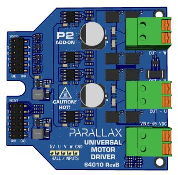
The open design and standard 0.1" connectors allow the Universal Motor Driver P2 Add-on Board to be used with other microcontrollers as well.
