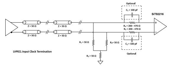
Figure 39 LVEPCL termination with hot swap protection
