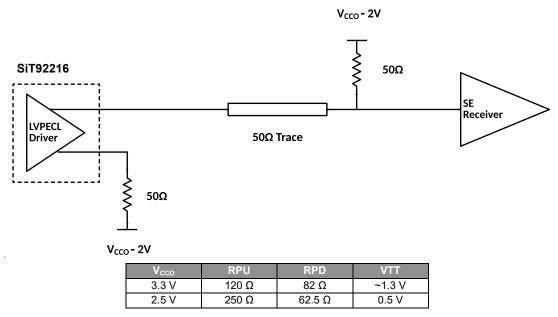
Figure 33 Termination scheme for DC coupled LVPECL, single ended
