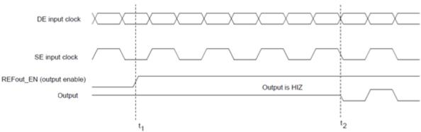
Figure 5 REF<sub>OUT</sub>\_EN: output enable
