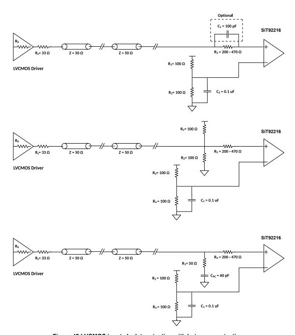
Figure 42 LVCMOS input clock termination with hot swap protection
