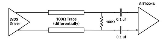
Figure 20 Termination scheme for AC coupled LVDS
