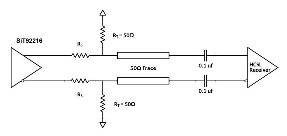
Figure 36 Output driver termination in HCSL AC coupled mode
