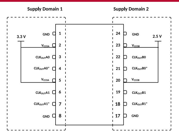
Figure 49: Multi Supply operation of SiT92216
