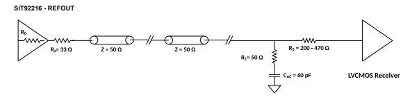
Figure 43 Different types of LVCMOS output clock termination with hot swap protection
