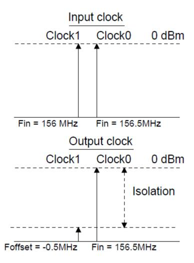
Figure 48 Parameter definition of isolation
