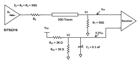
Figure 24 DC coupled LVCMOS output clock configuration - configuration 2
