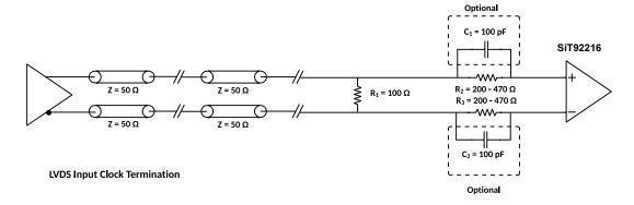
Figure 40 LVDS termination with hot swap protection
