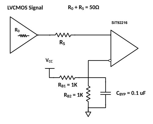
Figure 11: Direct coupling of LVCMOS clock to SiT92216
