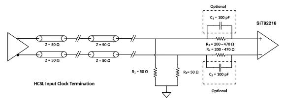
Figure 41 HCSL termination with hot swap protection
