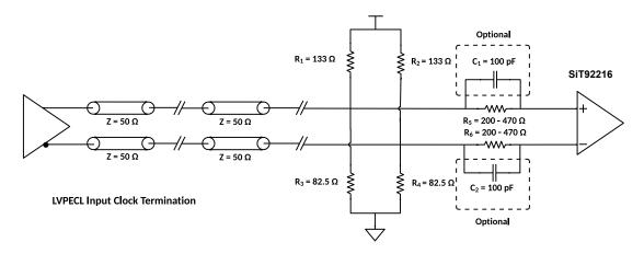
Figure 38 LVPECL termination with hot swap protection
