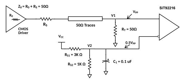
Figure 9 DC coupled LVCMOS input clock configuration - configuration 2
