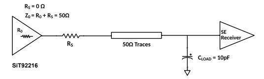
Figure 26 Typical application load
