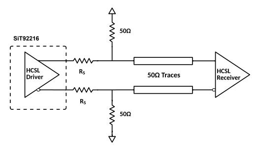
Figure 28 Termination scheme for DC coupled HCSL
