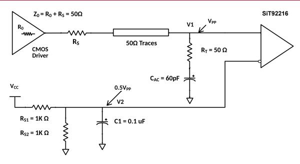
Figure 10 DC coupled LVCMOS input clock with series RC termination - configuration 3
