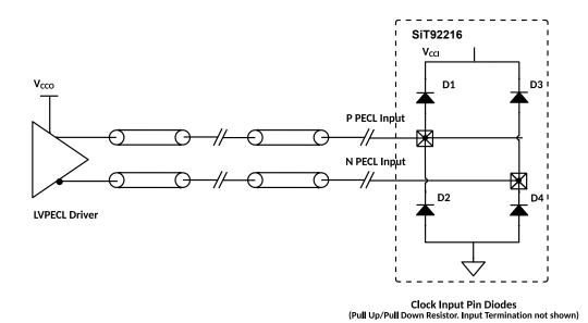
Figure 37 Typical input differential clock
