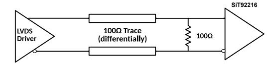
Figure 15 Termination scheme for DC coupled LVDS
