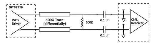
Figure 31 Termination scheme for AC coupled LVDS, driving LVDS receiver and CML receiver
