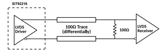
Figure 27 Termination scheme for DC coupled LVDS
