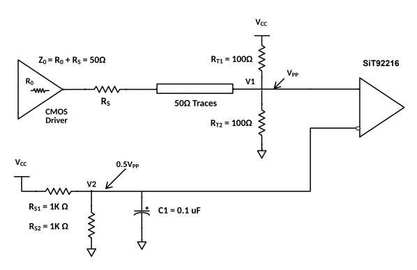
Figure 8 DC coupling of LVCMOS clock to SiT92216 – configuration 1
