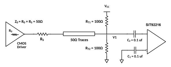
Figure 6 AC coupling LVCMOS clock to SiT92216
