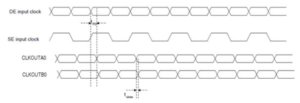
Figure 46 Parameter definitions of propagation delay and skew
