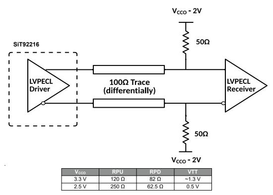
Figure 29 Termination scheme for DC coupled LVPECL
