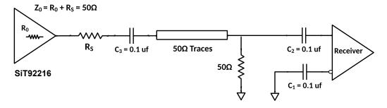
Figure 22 AC coupling of LVCMOS clock with single 50  $\Omega$  resistor termination to ground
