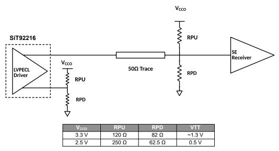
Figure 34 Termination scheme for DC coupled LVPECL, single ended, Thevenin equivalent
