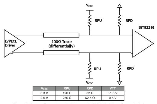
Figure 18 Termination scheme for DC coupled LVPECL, Thevenin equivalent
