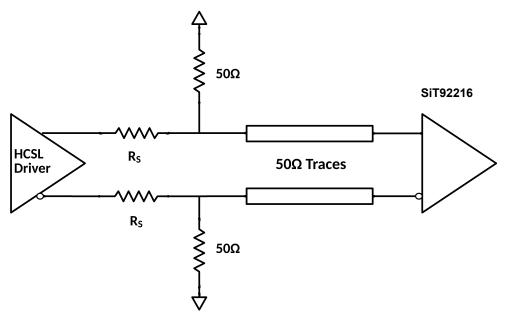
Figure 16 Termination scheme for DC coupled HCSL
