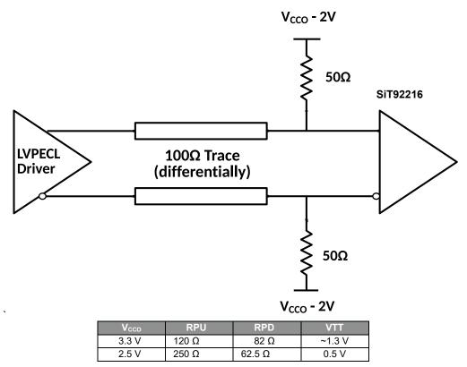
Figure 17 Termination scheme for DC coupled LVPECL
