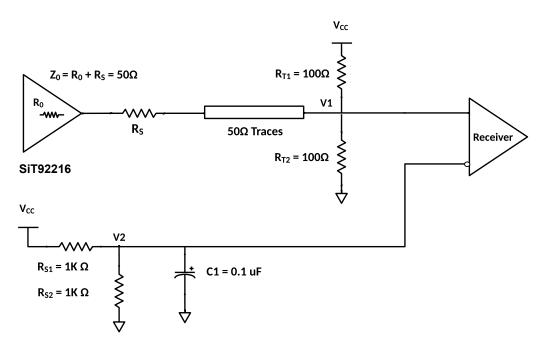
Figure 23 DC coupling of LVCMOS output clock termination - configuration 1
