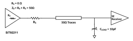
Figure 25 Typical application load
