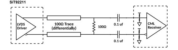
Figure 30 Termination scheme for AC coupled LVDS, driving LVDS receiver and CML receiver
