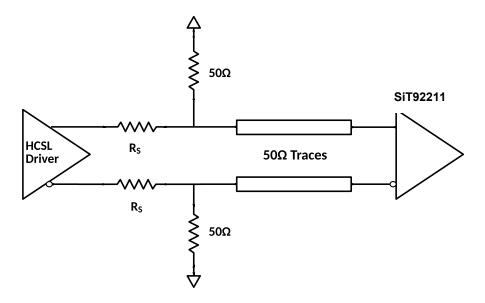
Figure 15 Termination scheme for DC coupled HCSL
