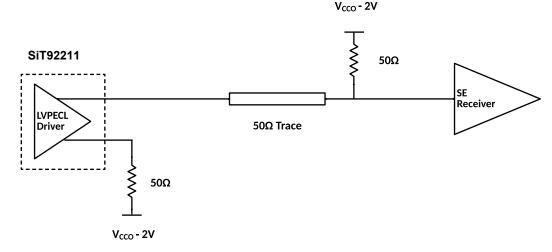
Figure 32 Termination scheme for DC coupled LVPECL, single ended
