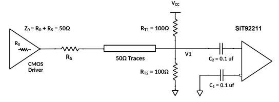
Figure 5 AC coupling LVCMOS clock to SiT92211
