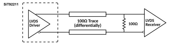
Figure 26 Termination scheme for DC coupled LVDS
