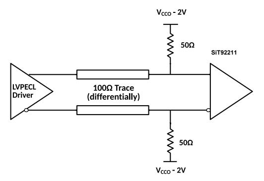
Figure 16 Termination scheme for DC coupled LVPECL
