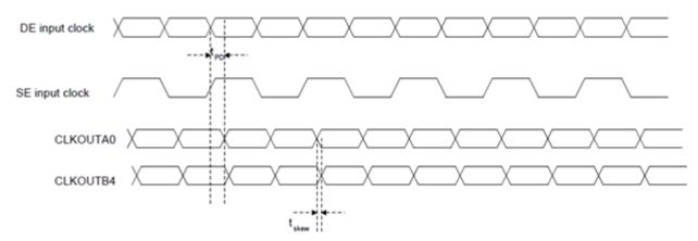
Figure 45 Parameter definitions of propagation delay and skew
