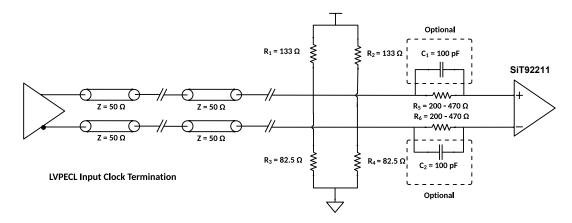
Figure 37 LVEPCL termination with hot swap protection
