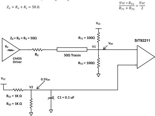
Figure 7 DC coupling of LVCMOS clock to SiT92211 – configuration 1
