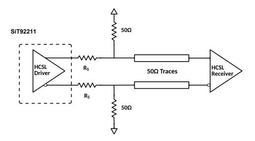
Figure 27 Termination scheme for DC coupled HCSL
