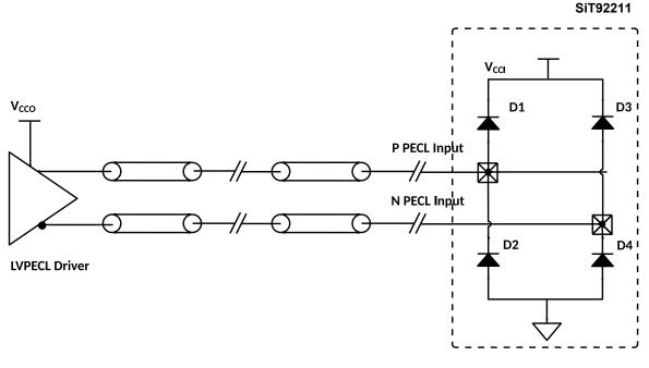
Clock Input Pin Diodes (Pull Up/Pull Down Resistor. Input Termination not shown)
