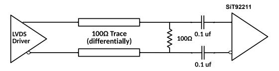
Figure 19 Termination scheme for AC coupled LVDS
