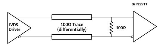
Figure 14 Termination scheme for DC coupled LVDS
