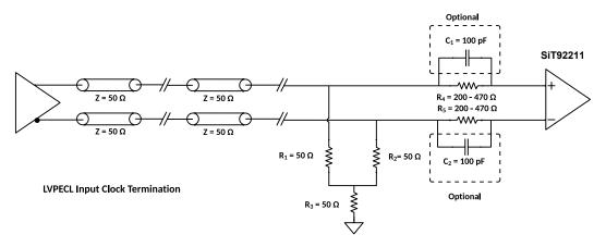
Figure 38 LVPECL termination with hot swap protection
