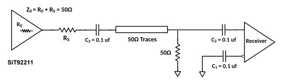
Figure 21 AC coupling of LVCMOS clock with single 50 Ω resistor termination to ground
