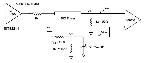
Figure 23 DC coupled LVCMOS output clock configuration – configuration 2
