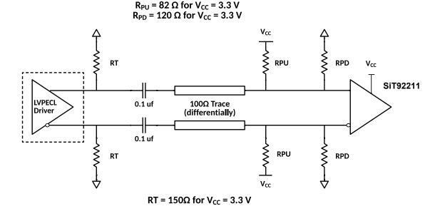
Figure 20 Termination scheme for AC coupled LVPECL, Thevenin Equivalent
