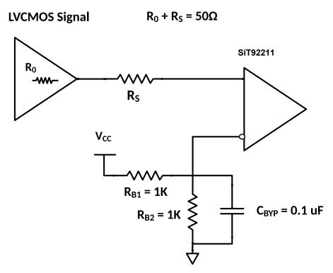
Figure 10: Direct coupling of LVCMOS clock to SiT92211
