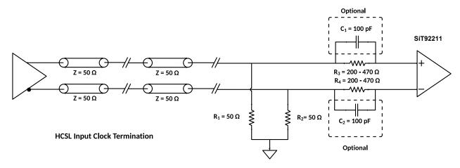
Figure 40 HCSL termination with hot swap protection
