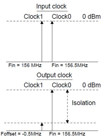
Figure 47 Parameter definition of isolation
