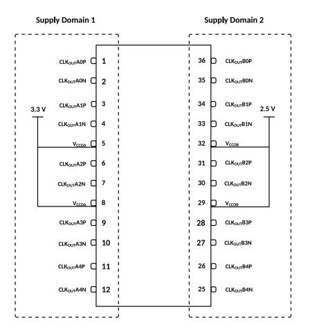
Figure 48: Multi Supply operation of SiT92211
