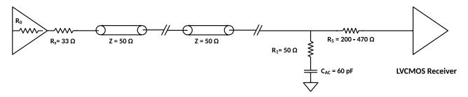
Figure 42 Different types of LVCMOS output clock termination with hot swap protection.
