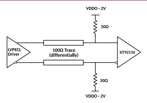
Figure 16 Termination scheme for DC coupled LVPECL.
