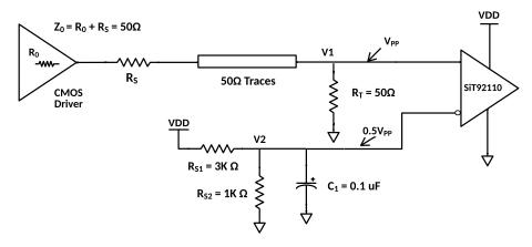
Figure 8 DC coupled LVCMOS input clock configuration – configuration 2
