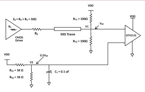
Figure 7 DC coupling of LVCMOS clock to SiT92110 - configuration 1
