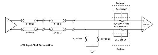
Figure 34 HCSL termination with hot swap protection
