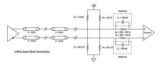
Figure 31 LVPECL termination with hot swap protection
