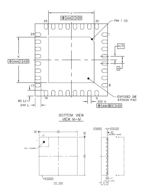
Figure 38 SiT92110 32 pin QFN package dimensions
