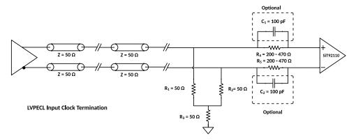
Figure 32 LVEPCL termination with hot swap protection
