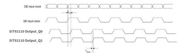
Figure 27 Parameter definitions of propagation delay and skew
