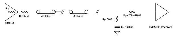
Figure 36 Different types of LVCMOS output clock termination with hot swap protection
