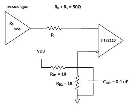
Figure 10: Direct coupling of LVCMOS clock to SiT92110
