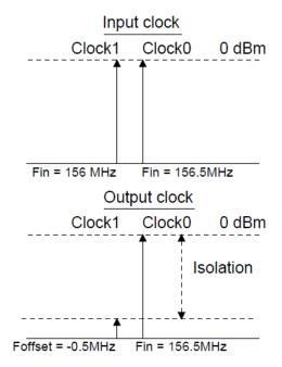
Figure 29 Parameter definition of isolation
