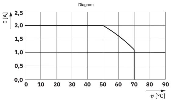
Maximum permissible current per path in uncoiled state
