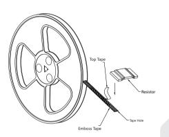
1. 4000 pcs. resistors are packed in a tape and wrapped in a reel.
