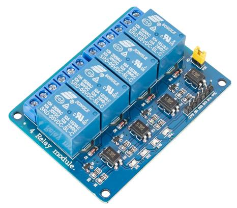
This is a LOW Level 5V 4-channel relay interface board, and each channel needs a 15-20mA driver current. It can be used to control various appliances and equipment with large current. It is equipped with high-current relays that work under AC250V 10A or DC30V 10A. It has a standard interface that can be controlled directly by micro-controller.
