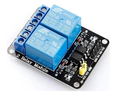
This is a LOW Level 5V 2-channel relay interface board, and each channel needs a 15-20mA driver current. It can be used to control various appliances and equipment with large current. It is equipped with high-current relays that work under AC250V 10A or DC30V 10A. It has a standard interface that can be controlled directly by micro-controller.
