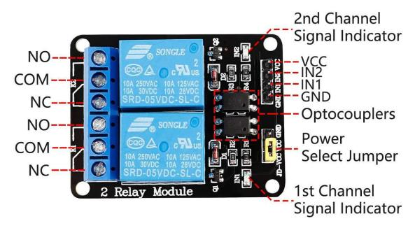
On the input side, where it receives the trigger signal, the connections typically include three or four pins, as outlined in the relay module circuit diagram:
