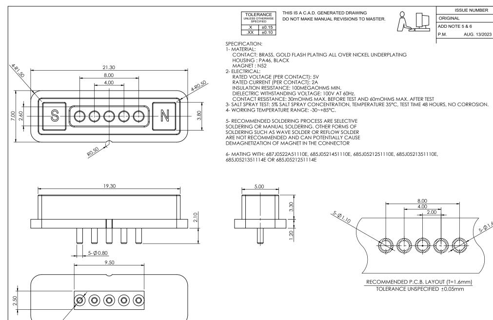
MAGNETIC SPRING LOADED CONNECTOR, 5POS, FEMALE
