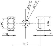
PCB LAYOUT LAYOUT TOLERANCE: ±0.05MM
