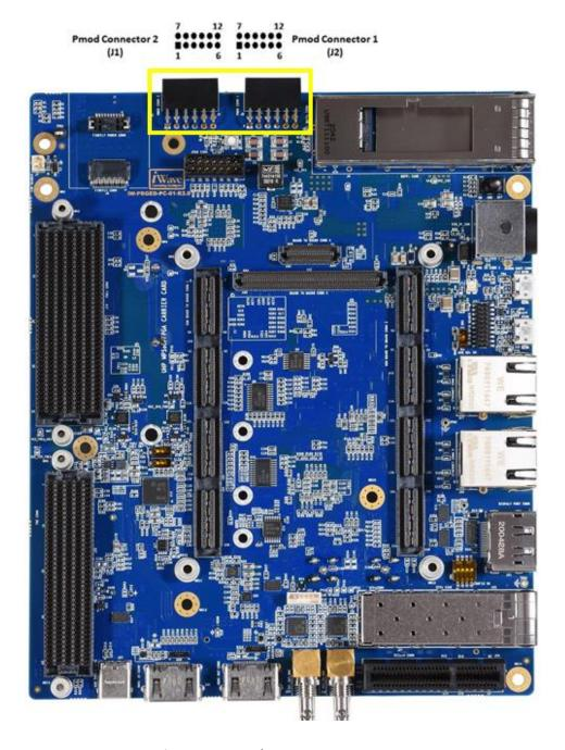
**Figure 21: Pmod Host Port Connectors**
