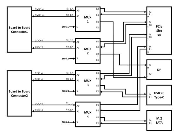
Figure 10: Transceiver Switch Connectivity.
