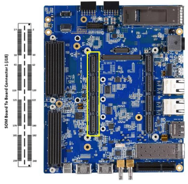
Figure 2: Board to Board Connector1
