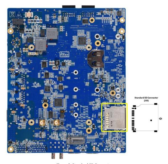
**Figure 8: Standard SD Connector**
