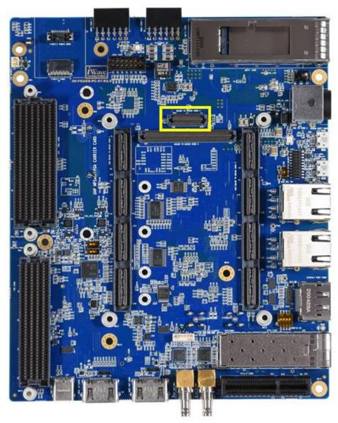
Figure 5 Board to Board Connector4
