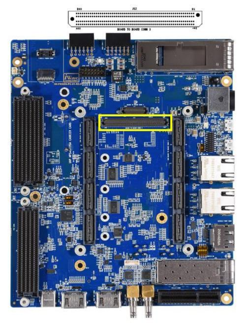
**Figure 4 Board to Board Connector3**
