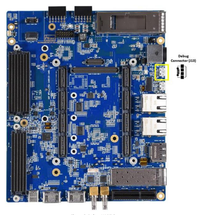
**Figure 9: Debug UART Connector**
