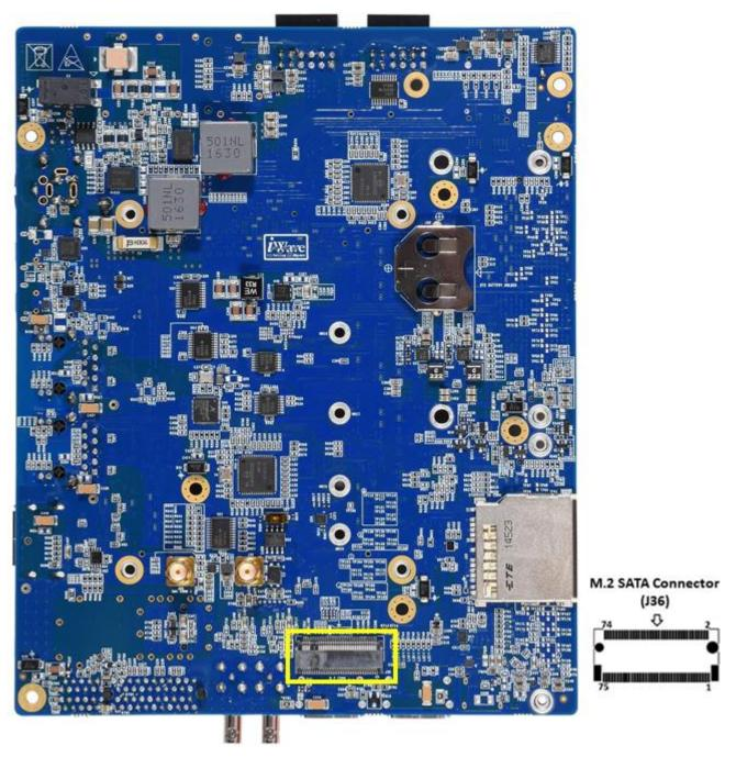
Figure 15: M.2 SATA Connector (Key M)
