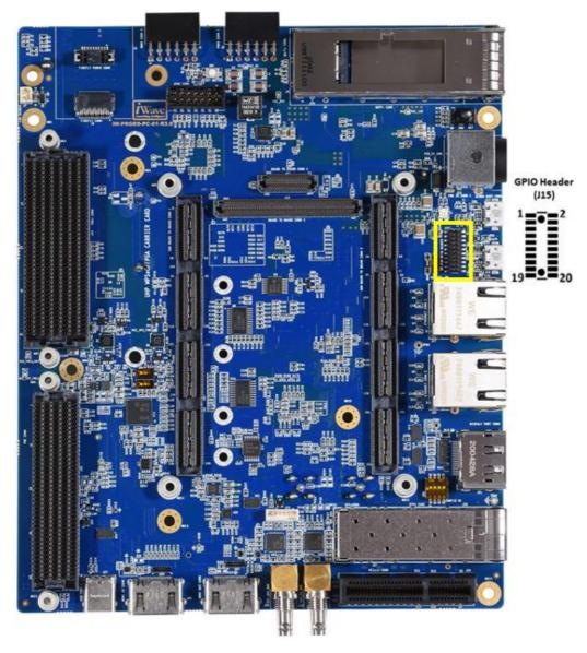
Figure 30: GPIO Header
