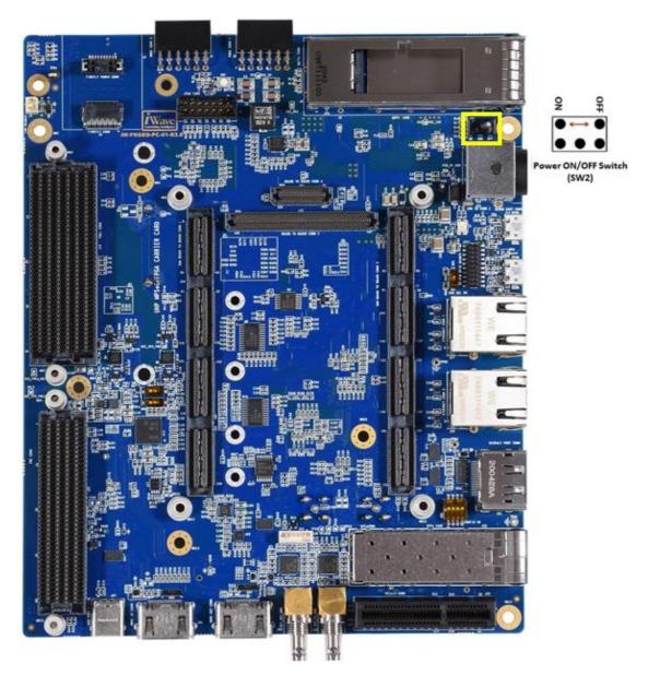
Figure 31: Power On/Off Switch
