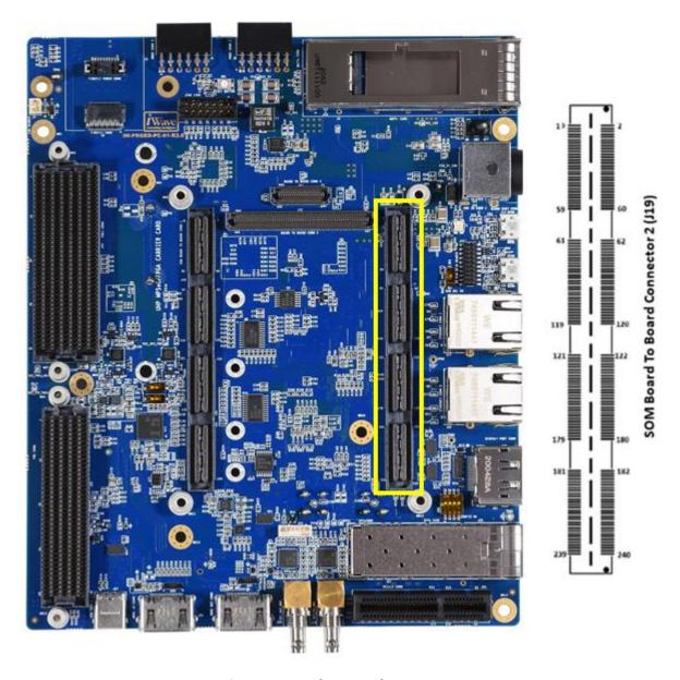
Figure 3: Board to Board Connector2
