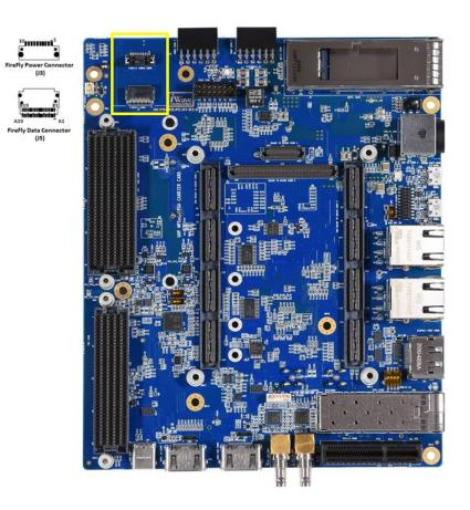
**Figure 20 FireFly Connector**
