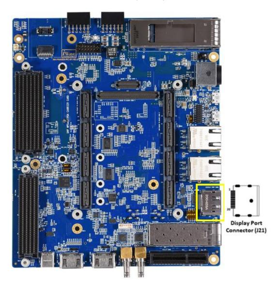
Figure 13: Display Port Connector
