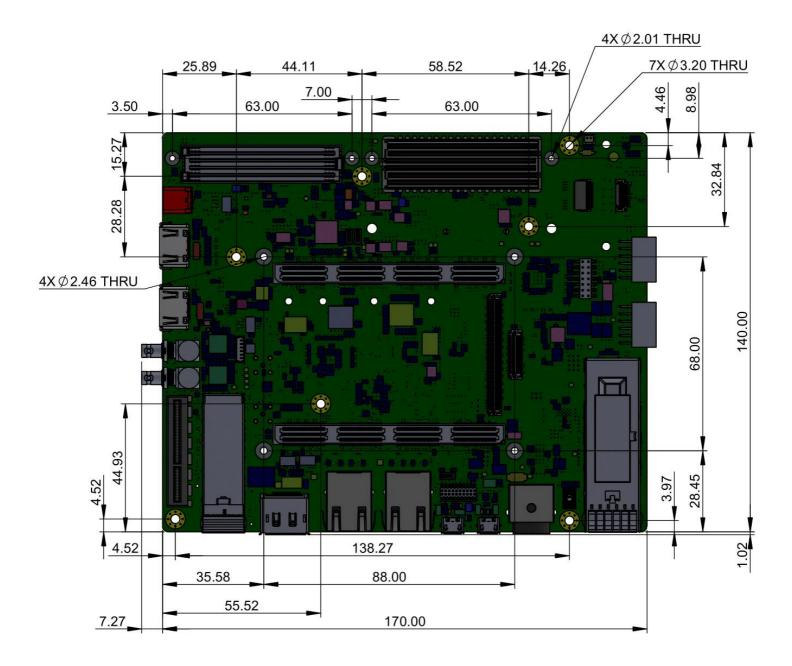
Figure 36: Carrier board Mechanical dimension - Top View
