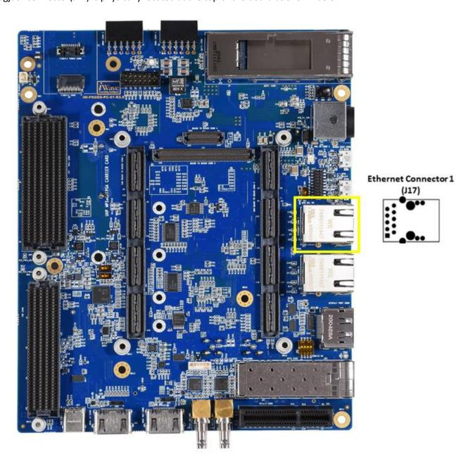
Figure 6: Gigabit Ethernet Connector1
