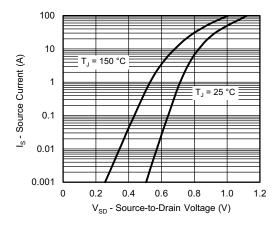
Source-Drain Diode Forward Voltage
