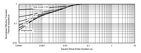
Normalized Thermal Transient Impedance, Junction-to-Case
