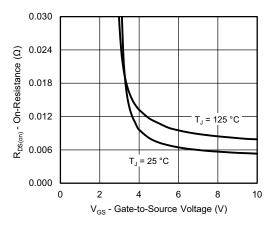
**On-Resistance vs. Gate-to-Source Voltage**
