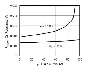
**On-Resistance vs. Drain Current**
