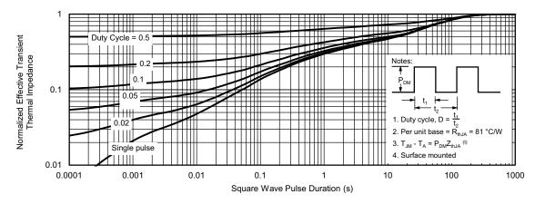
Normalized Thermal Transient Impedance, Junction-to-Ambient
