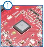
Clean application area on PCB with isopropyl alcohol and let dry before installation.
