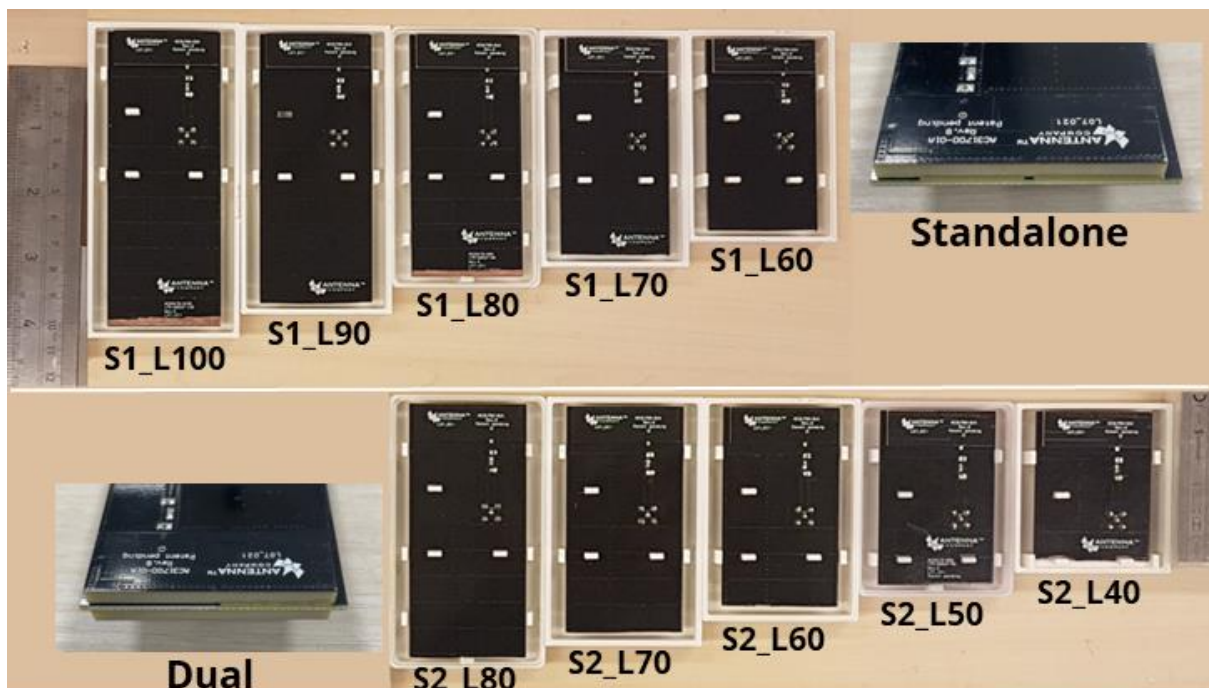
Figure 4: Overview of test boards used to characterize the AC31700-01A antenna (with and without additional booster element AC31700-01B)
