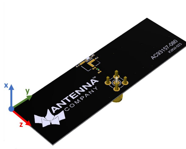
Figure 2: Illustration of radiation pattern evaluation planes
