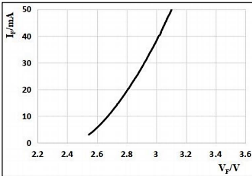
Figure 3. Forward Voltage Vs. Forward Current, I_F = f(V_F)
