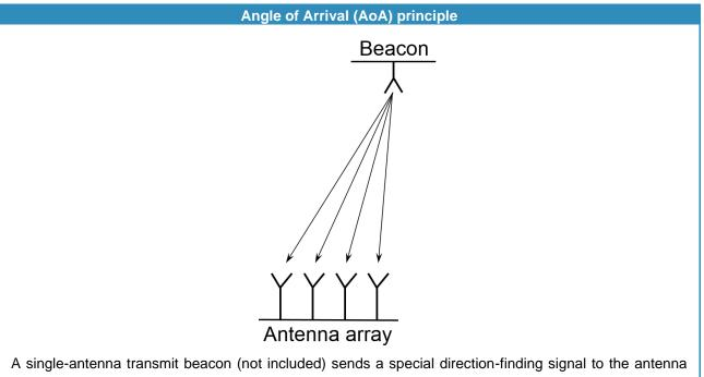
array. Angle calculation is based on phase information (phase differences) between the adjacent array antenna elements. The number of antennas in array affects the angle estimation accuracy. Bluetooth 5.x direction finding Angle of Arrival (AoA) protocol is supported by the following chipsets (not included): nRF5340, nRF52833, nRF52820, nRF52811 (Nordic Semiconductor), EFR32MG13, EFR32BG13, EFR32BG22, EFR32MG22 (Silicon Labs), CC2642, CC2652 (Texas Instruments),
