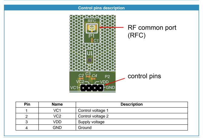
Control signals table for switching individual antennas in antenna array
