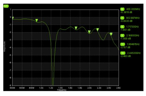
Figure 3: insertion losses of the AC20424-01
