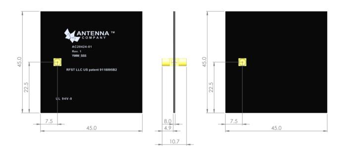
Figure 1: AC20424-01 visual representation and dimensions (in mm).
