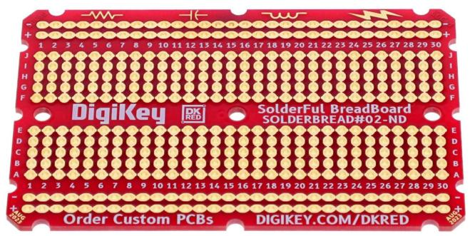
A Perfboard with a solderless breadboard format.
