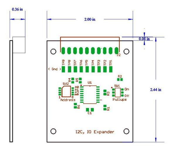
Please note: Side view only shows highest component above the module mounting surface.
