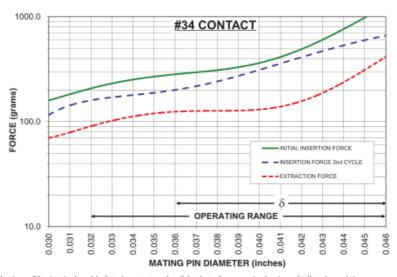
The insertion / extraction force characteristics above were derived using a 30 microinch gold-plated contact and polished steel gauge pins having a bullet-shaped tip.
