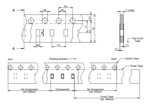
Figure 12: Tape packaging details of AC10300-01
