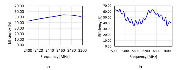
Figure 4: Efficiency of the AC10300-01. 2G efficiency (a) and 5G/6G efficiency (b)
