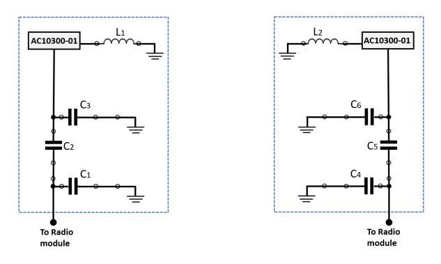
Figure 10: Required matching network topology for AC10300-01
