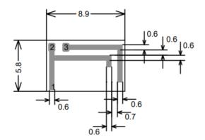
Figure 7: Footprint of the AC10300-01 on the top PCB layer. All dimensions are given in mm
