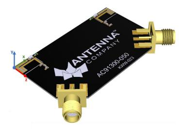
Figure 2: Illustration of radiation pattern evaluation planes
