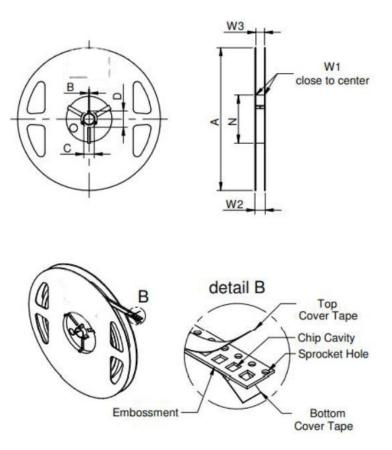
Figure 13: Reel packaging details of AC10300-01
