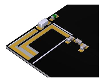
Figure 5: Isometric view of the AC10300-01 placement on the host PCB
