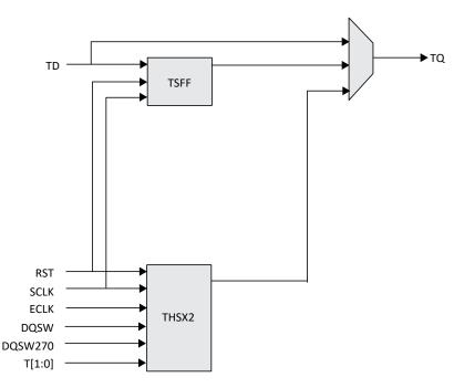
Figure 2.23. Tri-state Register Block on Bottom Side
