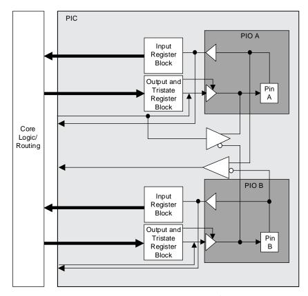
Figure 2.17. Wide Range Programmable I/O Cells
