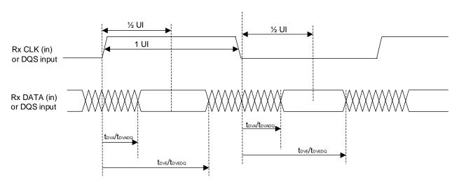
Figure 3.8. Receiver RX.CLK.Aligned and DDR Memory Input Waveforms
