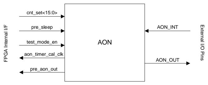
Figure 2.25. AON Functional Block Diagram
