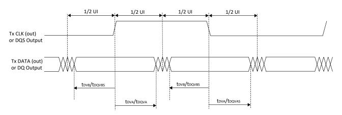
Figure 3.9. Transmit TX.CLK.Centered and DDR Memory Output Waveforms
