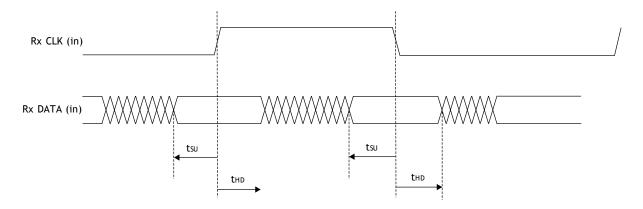
Figure 3.7. Receiver RX.CLK.Centered Waveforms
