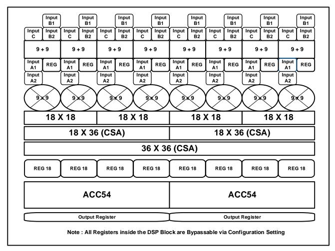
Figure 2.15. DSP Functional Block Diagram
