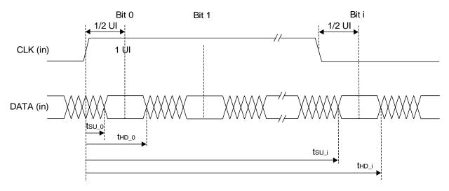
Figure 3.12. Receiver DDRX71\_RX Waveforms
