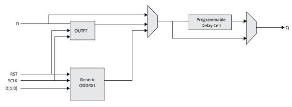
Figure 2.20. Output Register Block on Top Side
