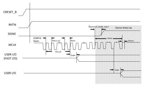
Figure 3.21. Master SPI Wake-Up Timing
