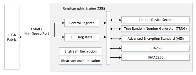
Figure 2.29. Cryptographic Engine Block Diagram
