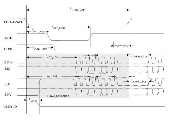
Figure 3.17. Slave SPI/I<sup>2</sup>C/I3C PROGRAMN Timing
