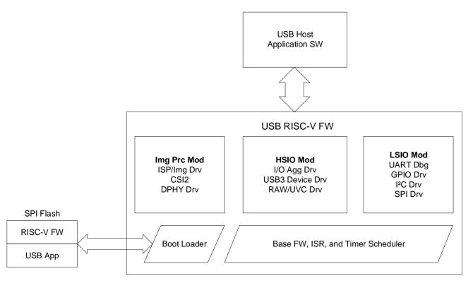
Figure 2.28. CrossLink-NX-33U USB RISC-V Host FW Stack
