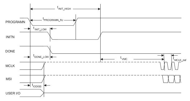
Figure 3.16. Master SPI PROGRAMN Timing
