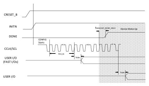
Figure 3.22. Slave SPI/I<sup>2</sup>C/I3C Wake-Up Timing
