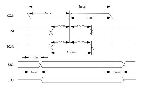
Figure 3.19. Slave SPI Configuration Timing
