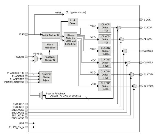
Figure 2.6. General Purpose PLL Diagram
