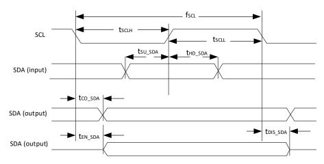
Figure 3.20. I<sup>2</sup>C /I3C Configuration Timing
