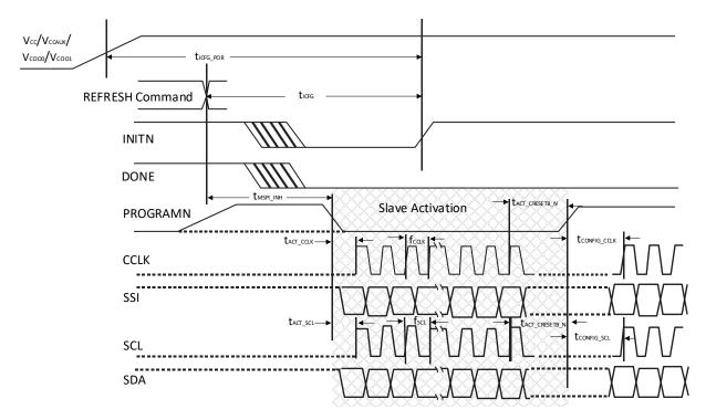
Figure 3.15. Slave SPI/I<sup>2</sup>C/I3C POR/REFRESH Timing
