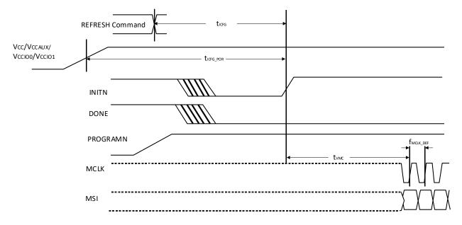
Figure 3.14. Master SPI POR/REFRESH Timing
