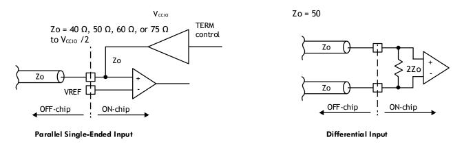
Figure 3.1. On-Chip Termination
