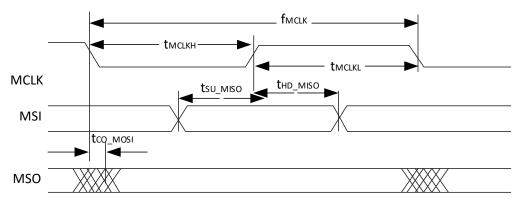
Figure 3.18. Master SPI Configuration Timing
