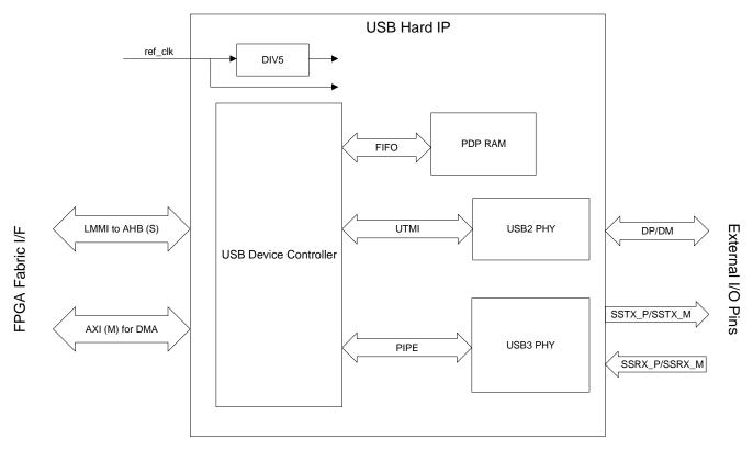
Figure 2.26. USB Hard IP Functional Block Diagram
