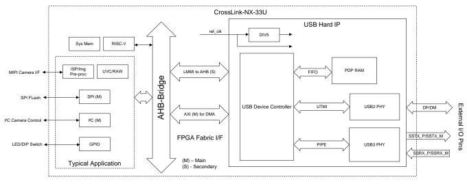
Figure 2.27. Typical USB Hardware Application Diagram
