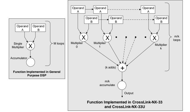
Figure 2.14. Comparison of General DSP, CrossLink-NX-33, and CrossLink-NX-33U Approaches
