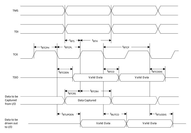
Figure 3.23. JTAG Port Timing Waveforms
