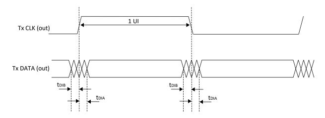
Figure 3.10. Transmit TX.CLK.Aligned Waveforms
