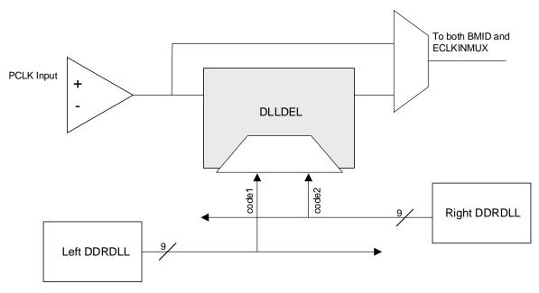
Figure 2.11. DLLDEL Functional Diagram
