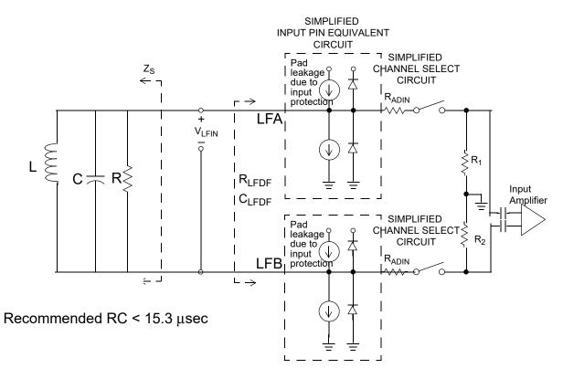
Figure 122. LFR Detector Input Equivalent Circuit
