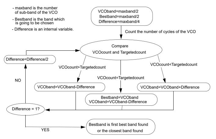
Figure 112. VCO Calibration State Machine
