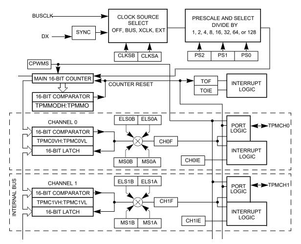
Figure 42. TPM1 Block Diagram
