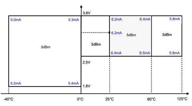
Figure 123. Dynamic Power Adjustment - 315 MHz
