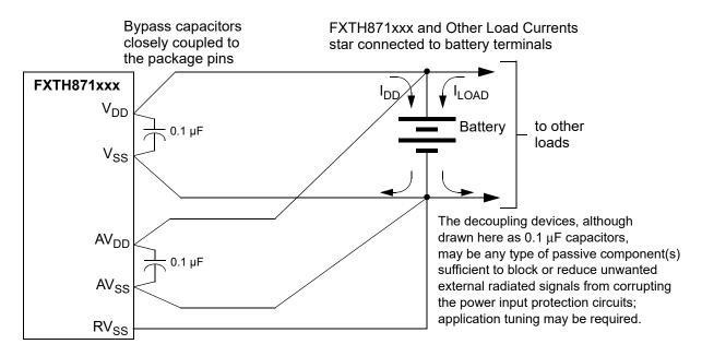
Figure 6. Recommended Power Supply Connections
