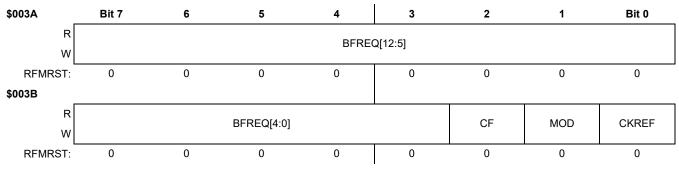
Figure 108. PLL Control Registers B (PLLCR[3:2], RPAGE = 0)
