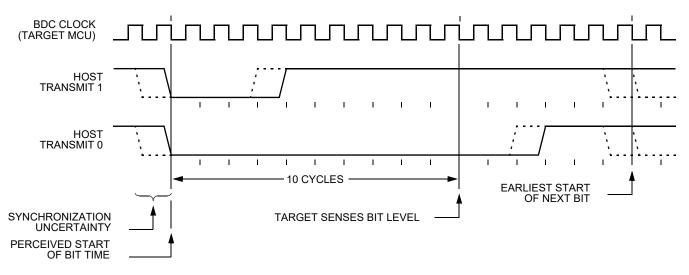
Figure 115. BDC Host-to-Target Serial Bit Timing
