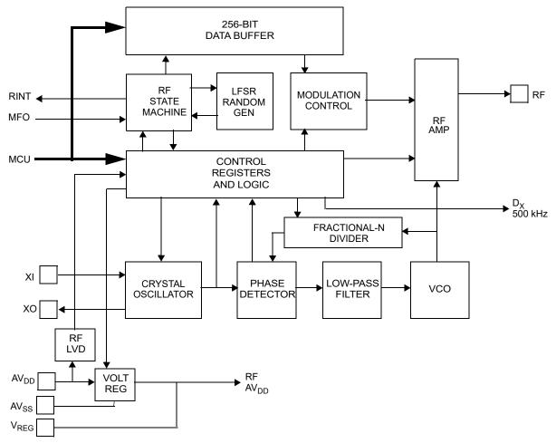
Figure 89. RF Transmitter Block Diagram
