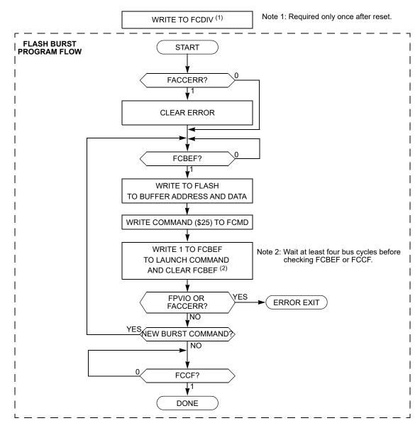
Figure 10. FLASH Burst Program Flowchart
