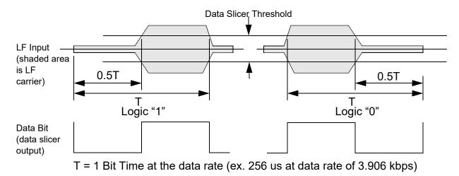
Figure 67. Manchester Encoded Datagram for LFPOL = 0
