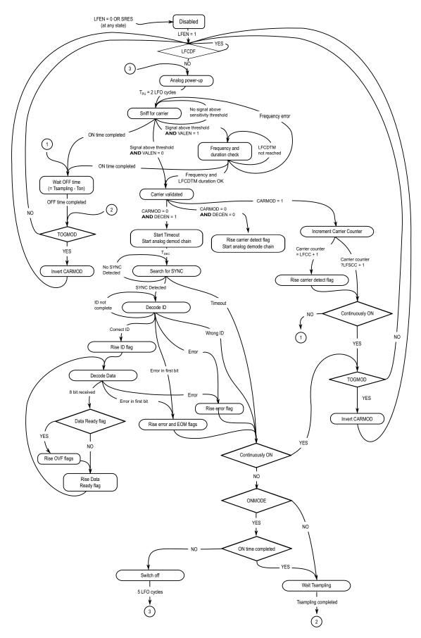
Figure 66. FXTH871x6 LFR State Machine Diagram
