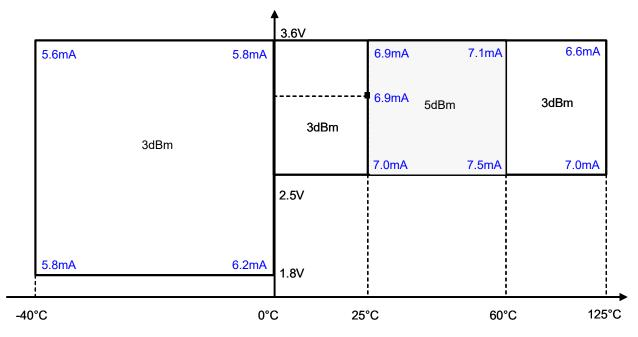
Figure 124. Dynamic Power Adjustment - 434 MHz
