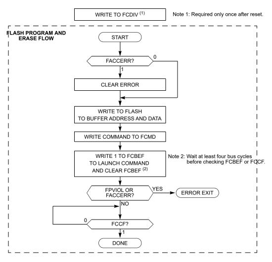
Figure 9. FLASH Program and Erase Flowchart
