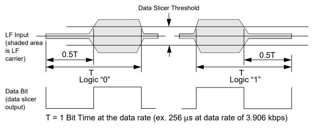
Figure 68. Manchester Encoded Datagram for LFPOL = 1
