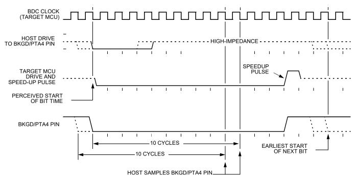
Figure 117. BDM Target-to-Host Serial Bit Timing (Logic 0)
