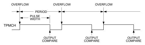
Figure 54. PWM Period and Pulse Width (ELSnA = 0)
