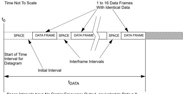
Space Intervals have No Carrier Frequency Output, equivalent to Data = 0 and may have the RFM crystal oscillator, VCO and PLL turned off by the IFPD bit.
