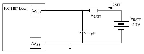
Figure 126. Battery Performance Test Configuration
