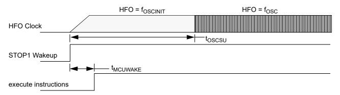
Figure 120. MCU Startup Delays
