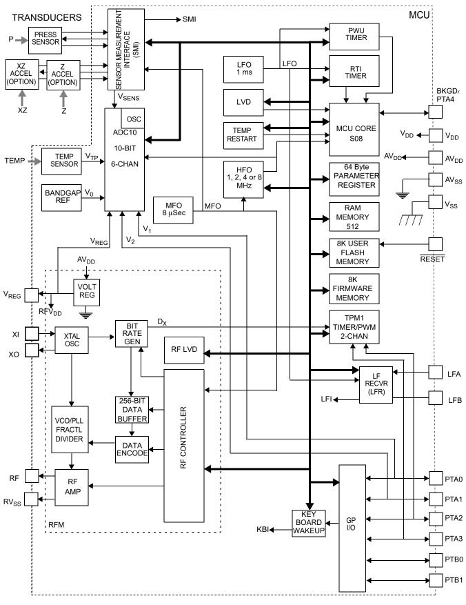
Figure 1. FXTH871x6 Overall Block Diagram
