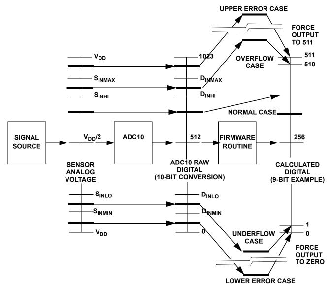
Figure 113. Measurement Signal Range Definitions
