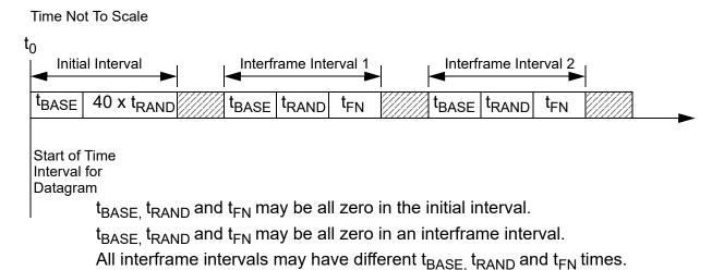
**Note:** If  $t_{BASE}$  and  $t_{FN}$  are both set to non-zero, and  $t_{RAND}$  is set to 0, the system will decrement both  $t_{BASE}$  and  $t_{FN}$  simultaneously rather than serially, such that the effective Interframe Interval will be equal to the larger of  $t_{BASE}$  or  $t_{FN}$  settings.
