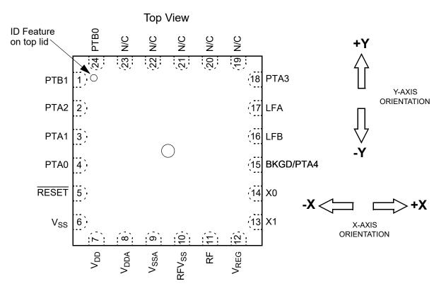
N/C = No Connect: Do not connect PCB pads to signal traces, power/ground or multi-layer via.
