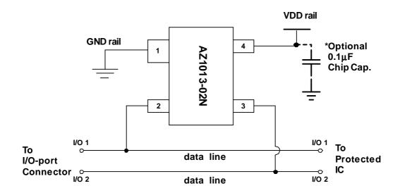
Fig. 2 Data lines and power rails connection of AZ1013-02N.
