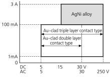
Note) If the contact is being used in the constant low-level circuit load range, the Au-clad double layer contact type is recommended. If there is a danger of the current being less than 0.5 A, for instance if the contact is being turned on and off, the Au-clad triple layer contact type is recommended.
