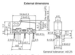
Note) As for the dimensions of lever types, dimensions other than terminals are same as P/C board terminal.
