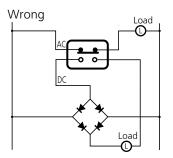
3) Avoid circuits which apply voltage between contacts. (This may lead to mixed deposition.)
