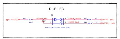
Figure 10. RGB schematic diagram
