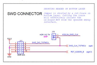
Figure 5. SWD debug connector to K32L2A
