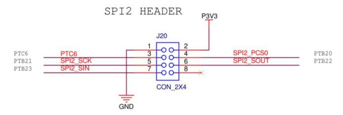
Figure 13. Header SPI2 Header
