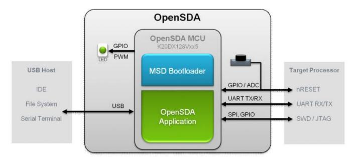
Figure 4. OpenSDA block diagram
