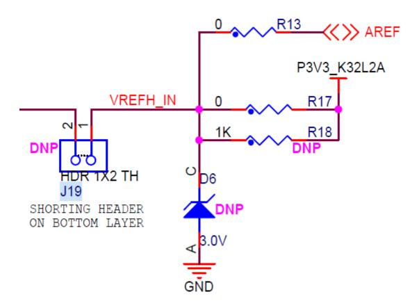
Figure 14. VREFH circuit schematic
