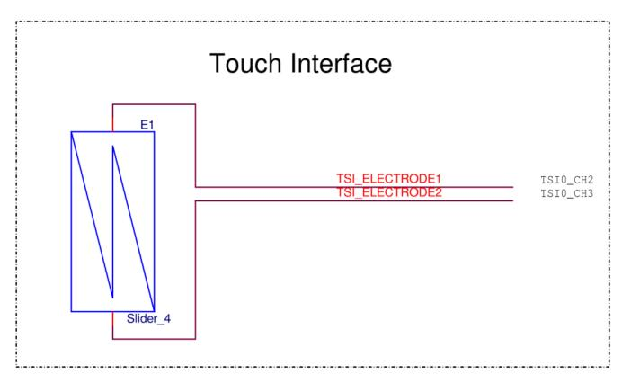
Figure 7. Touch slider connection
