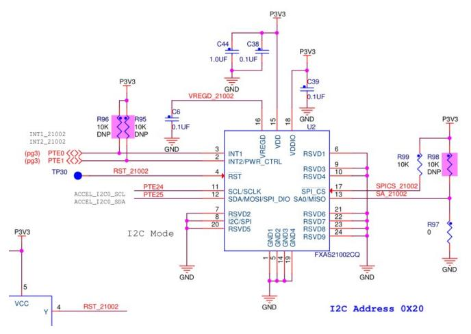
Figure 9. FXAS21002C schematic diagram
