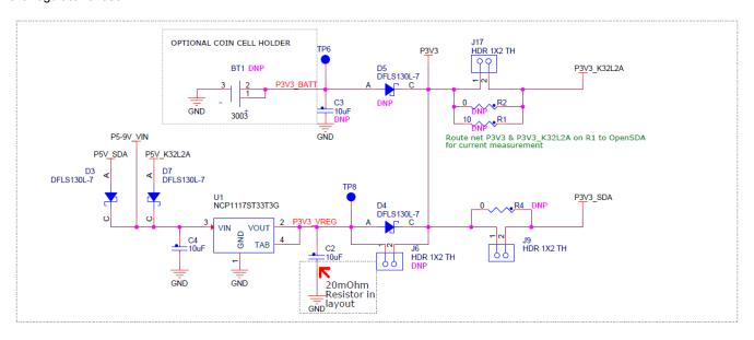
Figure 3. Power supply schematic
