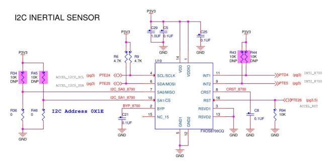
Figure 8. FXOS8700CQ schematic diagram
