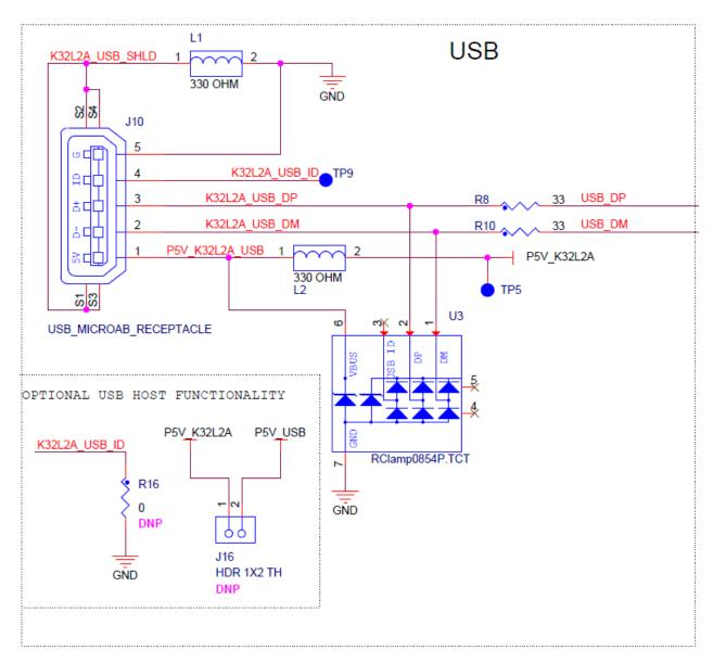
Figure 6. USB connector schematic
