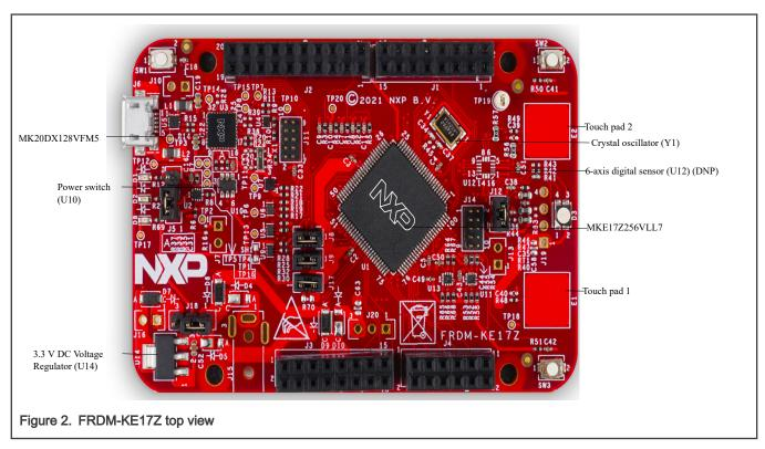
The figure below shows the onboard jumpers and connectors on FRDM-KE17Z.
