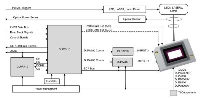
Figure 2. DLPR410 and DLPC410 with DMD Example Block Diagram
