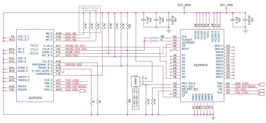
Figure 1. DLPC410 and DLPR410 Connection Schematic
