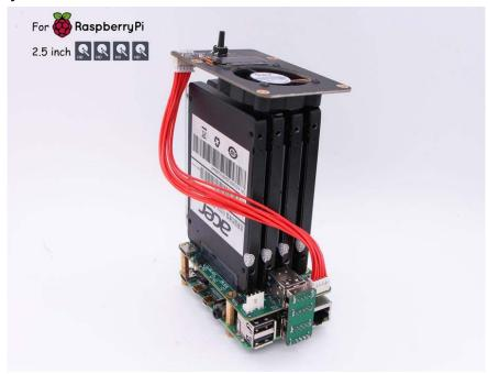
The Dual SATA HAT utilizes two high-performance JMS561 (one JMS561 for the Dual SATA HAT) and provides up to 400MB/s read/write performance with four disks in RAID0 mode.
