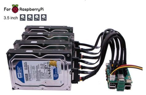
For 2.5inch HDD setups, the USB PD/QC power adapter ( >=30W power adapter ) is sufficient to power the disk drives and the Raspberry Pi 4 together. It is important to mention that the power connector on the SATA HAT must be used to power up the NAS with Raspberry Pi 4.
